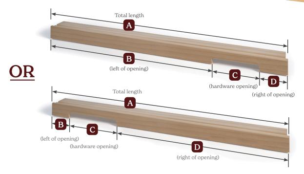
Whether your hardware opening is oriented on the left OR right, ensure you measure B, C, and D from the left to right when facing the front of the sill stop (see diagram above).
